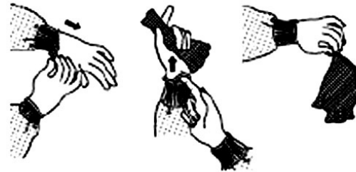
Take off gloves carefully, turn them inside out.
